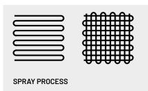
Start with the spraying outside the painting surface and apply several thin layers evenly in a "cross coat".
